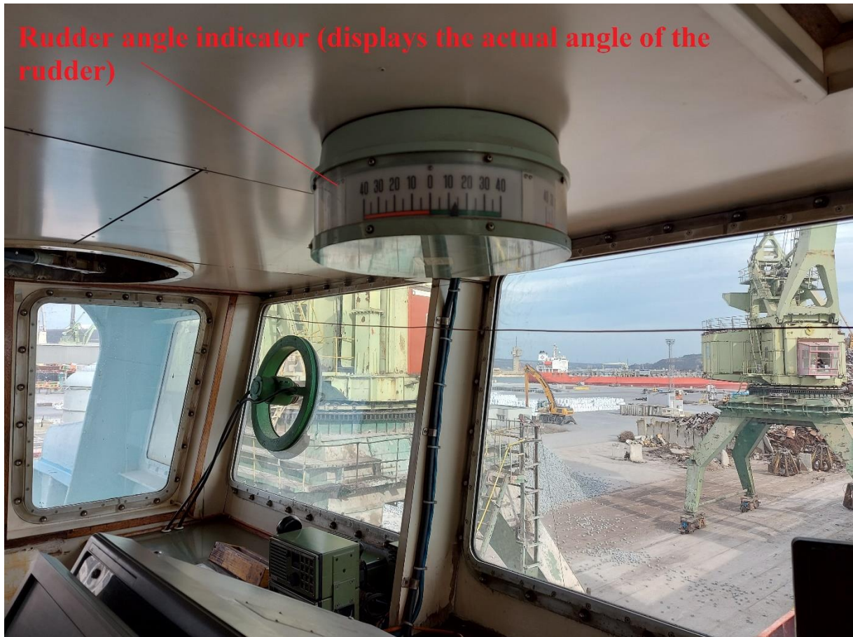
Figure 6 – Rudder angle indicator on the bridge ceiling
