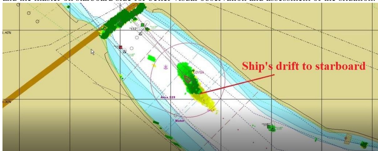
Figure 7 – Radar image showing the ship’s drift to starboard (points behind the ship are her past track)
