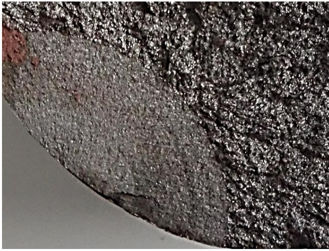
Fig.55. Fatigue grooves in zone A (OM)
